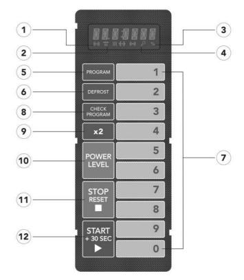
NOTE: The oven can be programmed for a maximum of 20 minutes at 100% power, and 60 minutes if 80% power or less is selected.
