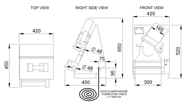
Nota: The dimensions indicated in the views are in millimeters
